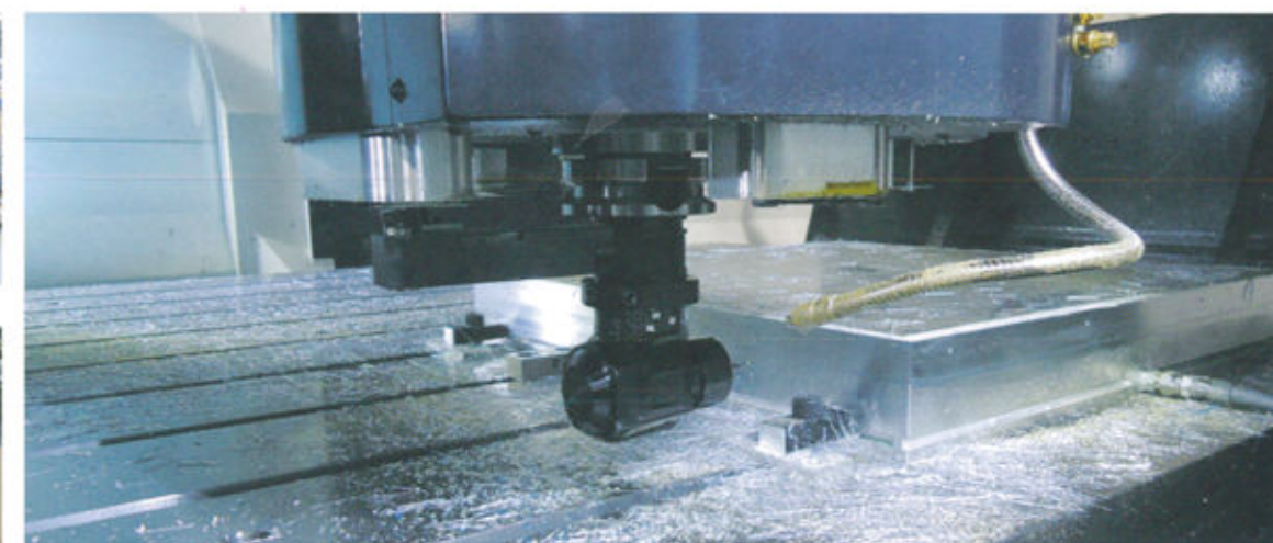
Side surface cutting by FJV-100/120 II with angle tool
